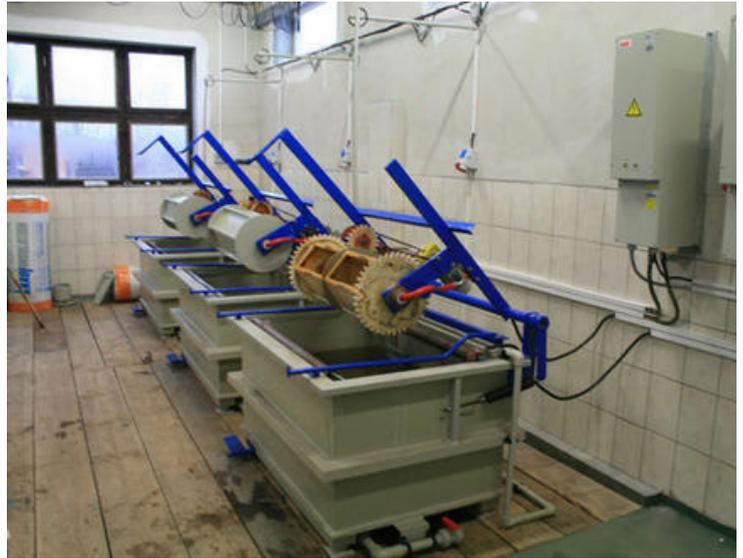
Barrel plating is a process of electroplating large quantities of smaller parts at once. This method of plating is most common among people whose plating project specification is very complicated and where a project must follow a stringent guideline for testing or meet the standards which the industry has in place for metal plating.
