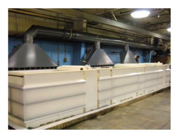
Therefore, if you are using plastic plating tank, you must make sure that there are adequate protection and regular maintenance of these tanks to prevent a fire hazard. Don't forget, when there is a fire from the plastic plating tank, other parts around like plastic piping and ductwork will also catch fire and spread it to other areas.
