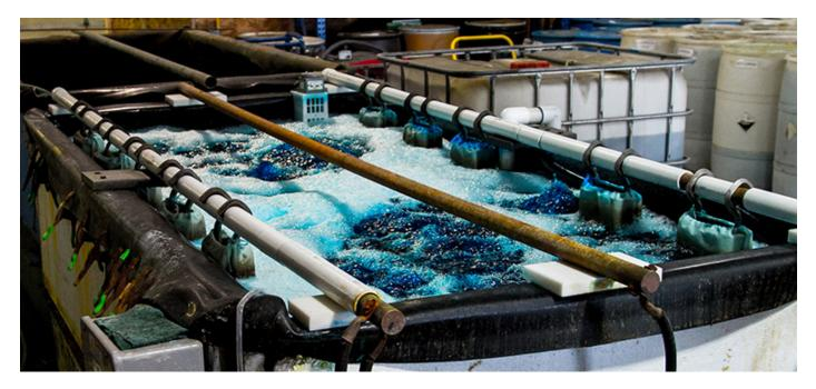
There are two methods of plating which is predominant in the industry, barrel plating, and rack plating. You can use both methods to plate both metals and plastic materials. No matter the method you want to use, there is need to consider the plating tank in which either the rack or barrel resides.
