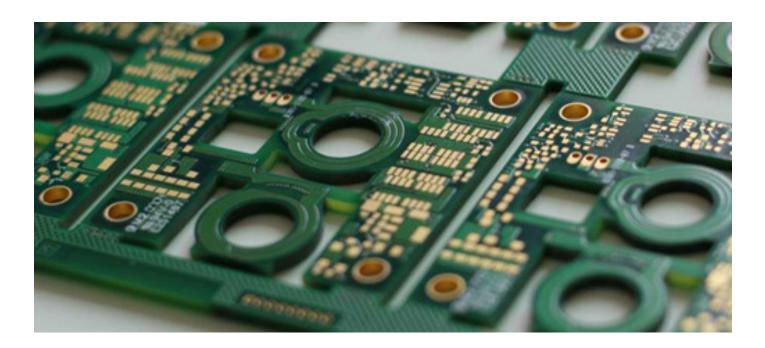
Printed circuit boards serve as a platform for connecting several electronic components. The material of the PCB card does not conduct electricity like plastic or fiberglass. When you look closely at a printed circuit board, you will notice some thin lines of copper inside it or on the board's surface. These thin lines between the layers of plastic are responsible for directing electricity through the board to the right places where it is necessary.
