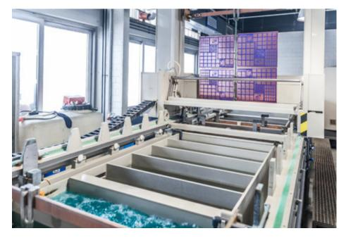
This technology behind this process is called PCB manufacturing and it describes a type of plating or its protruding part. The process of this plating method is:
