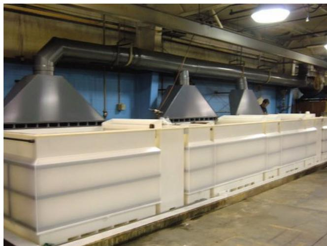
Therefore, if you are using plastic plating tank, you must make sure that there are adequate protection and regular maintenance of these tanks to prevent a fire hazard. Don't forget, when there is a fire from the plastic plating tank, other parts around like plastic piping and ductwork will also catch fire and spread it to other areas.
