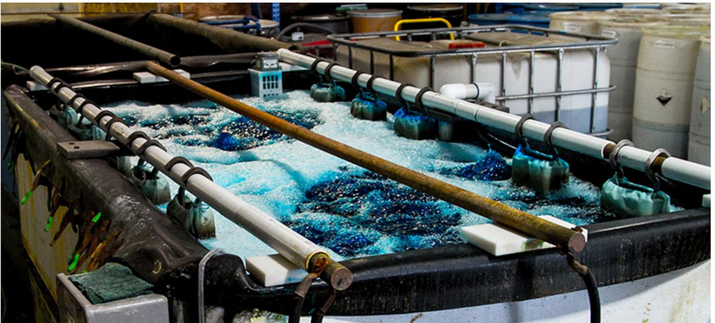
There are two methods of plating which is predominant in the industry, barrel plating, and rack plating. You can use both methods to plate both metals and plastic materials. No matter the method you want to use, there is need to consider the plating tank in which either the rack or barrel resides.
